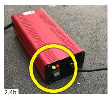
Always disconnect the mains supply before disconnecting the battery. Don't forget to replace Bugzi's power lead after charging!
