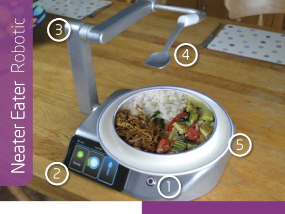
The Neater Eater® Robotic enables people to feed themselves. It is simple to use, controlled by a touchscreen or plug-in switches. Touchscreen menus and help guide demonstrate many options such as setting the mouth position, automatic spoon-wiping and plateturning. There are fork and snackholder modes and a routine to scrape the plate at the end of the meal.
