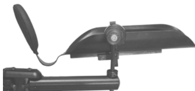
Slide positioned so forearm support is balanced.
