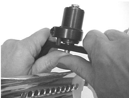
Pressing out pivot pin with thumbs.
