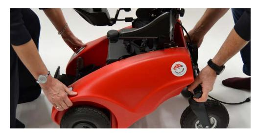
See above picture for lifting Wizzybug. It is a **2 person** lift. Never lift by the headrest or armrests. Instead use the front wheel arches and black back metal beam.
