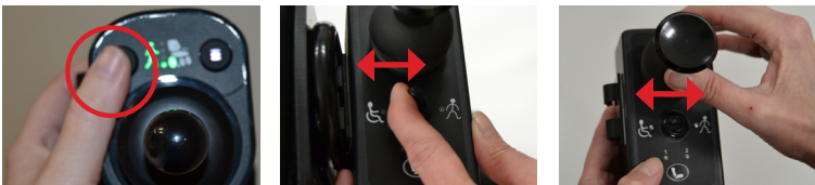
Fig 38 Switch between child use and carer use by pressing the ON/OFF button on the carer control (for a LiNX) or flicking the switch on carer control (for a Shark or DX)
