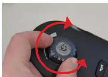
36 Fig 34 LiNX speed dial
