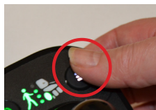
Fig 35 LiNX carer control speed button
