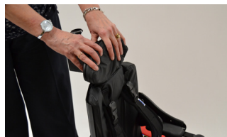
Fig 44 Pull Wizzybug by the headrest, with wheel releases disengaged to transport
