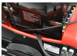
Fig 29 Storing excess cables
